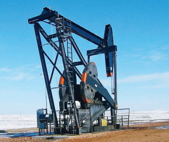
ENCORE'S PUMPING UNIT PULLS OIL FROM A MILE BELOW GROUND.
